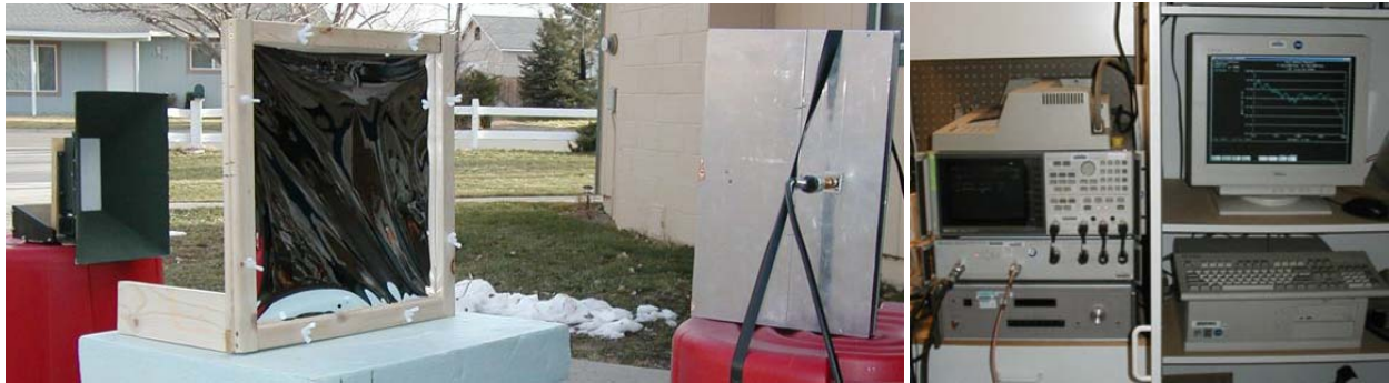
Figure 7: Test setup (emitter feed horn (left), sample under test (middle), and receiver antenna (right)) and computer controlled network analyzer used for RF measurements
