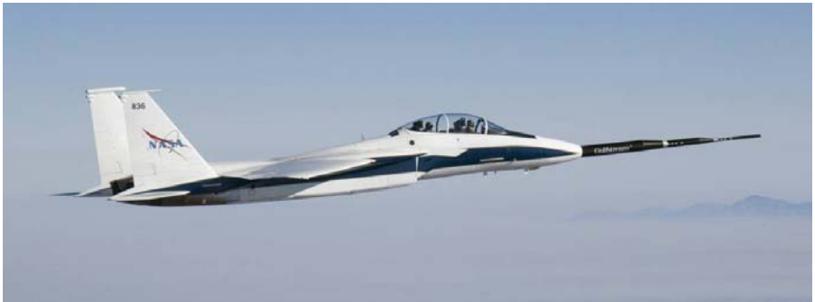
Figure 4. NASA F-15B modified with Gulfstream Aerospace Quiet Spike™ (shown in the fully extended position).
