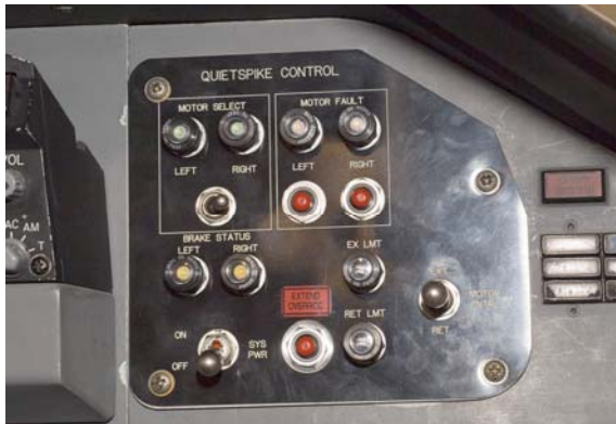
Figure 6. Quiet Spike control panel in the rear cockpit.
