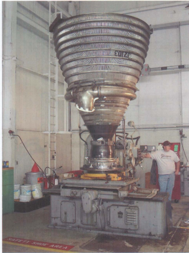
Figure 7. Heritage J-2 undergoes power pack preparations.
