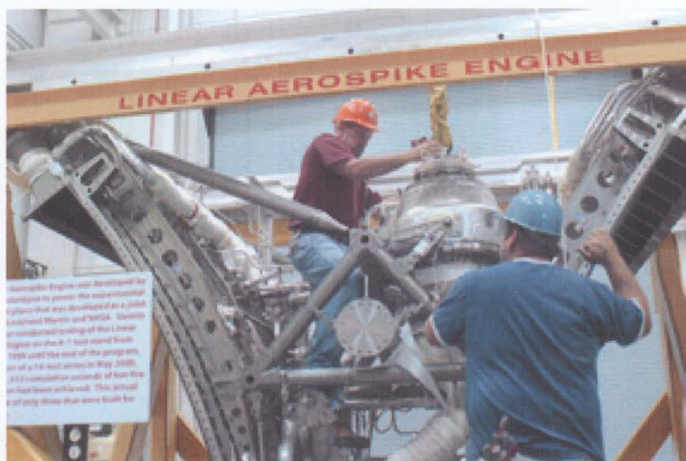
Figure 5. X-33 aerospike engine turbomachinery removal at Stennis Space Center.
