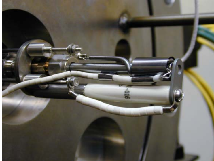
Figure 6.—Cathode assembly mounted in vacuum facility; Pt-Rh thermocouple attached.
