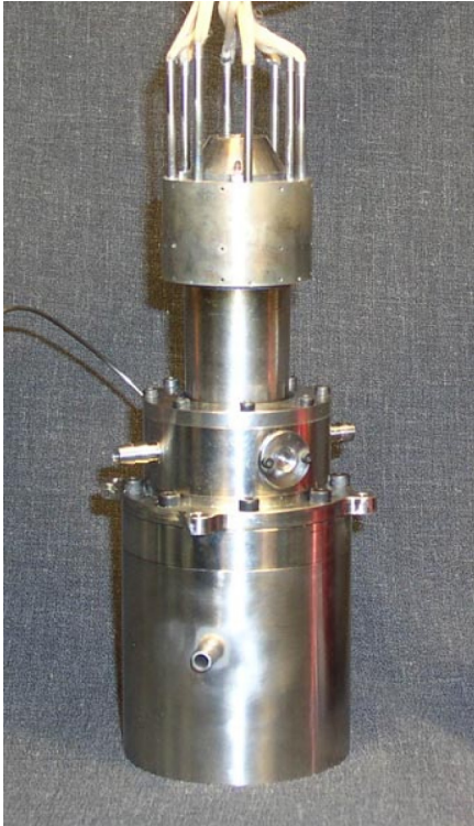
Figure 1.—Sunpower Frequency Test Bed Stirling convertor.
