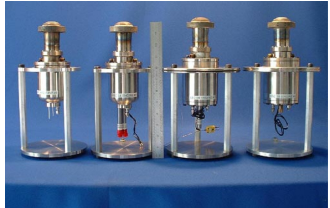
Figure 2.—Four nonhermetically sealed advanced Stirling convertors (ASC-1s).
