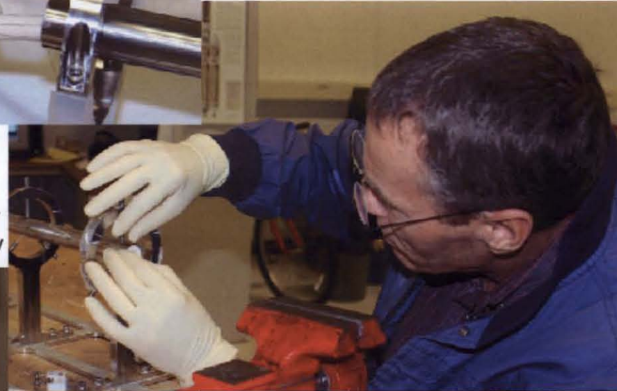
Insertion of insulator into sheath assembly
