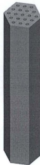
Figure1: Geometry of a 19-channel flow element
