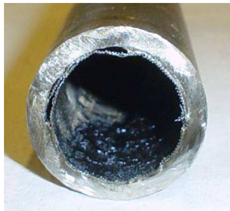
Figure 12. Picture of Therminol/stainless steel life test pipe taken off life test after 300 hours at 450°C.
