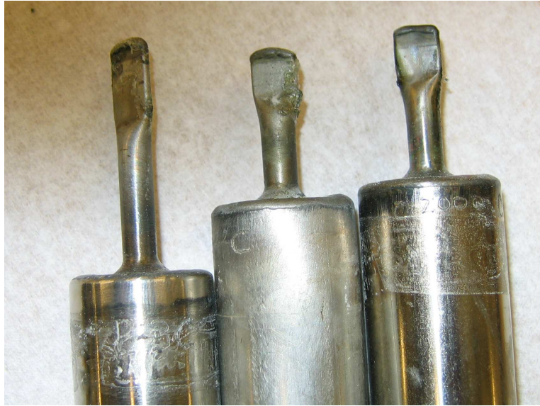
Figure 6. The GaCl 3 heat pipes leaked at the pinch-off after one week. Note that all of the pinch-offs used C-22 tubing.
