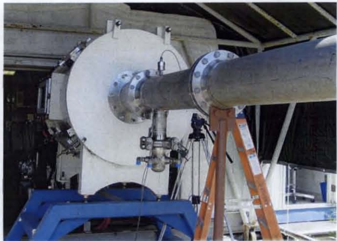
Figure 16. Installed test section and ejector pump.
