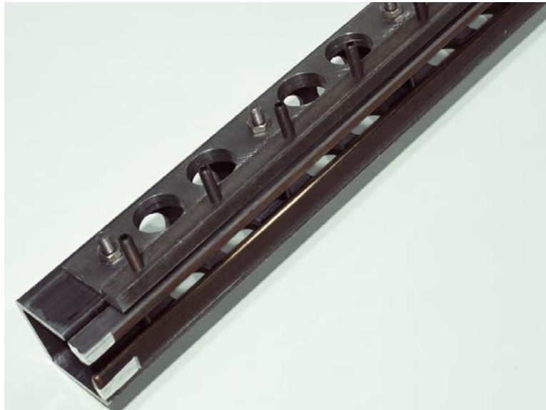
Figure 9. Vertical edge test fixture.
