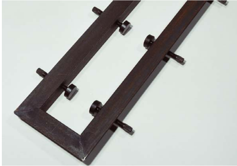
Figure 10. Horizontal edge test fixture.
