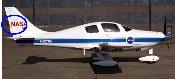
Figure 3: Lancair Columbia 300 aircraft and NAV antenna located on tail (blue ellipse).
