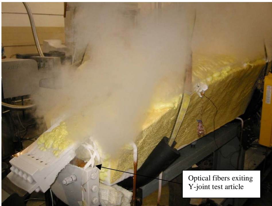
Figure 7. Installed Y-joint test article undergoing cryogenic cooling. Liquid Helium is sprayed onto the Y-joint dome surface and released to the atmosphere.
