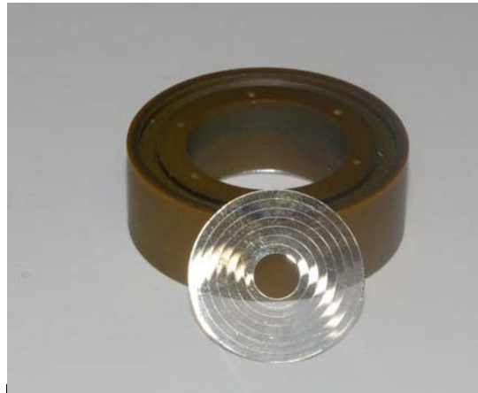
Disk Leaning Against Outer Fixture Housing
