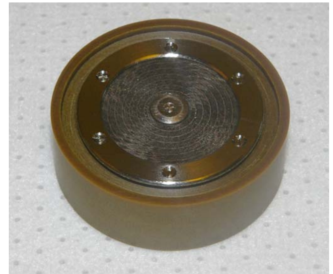
Assembled Oscillating-Flow-Rig Test Fixture (Stack of 42 Disks)
