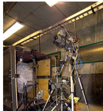
Figure 3.—Three-dimensional digital image correlation system setup.
