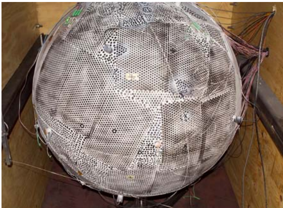
Figure 2.—COPV dot pattern painted on vessel for digital image correlation.
