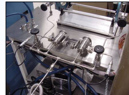
Gas Management Manifold
