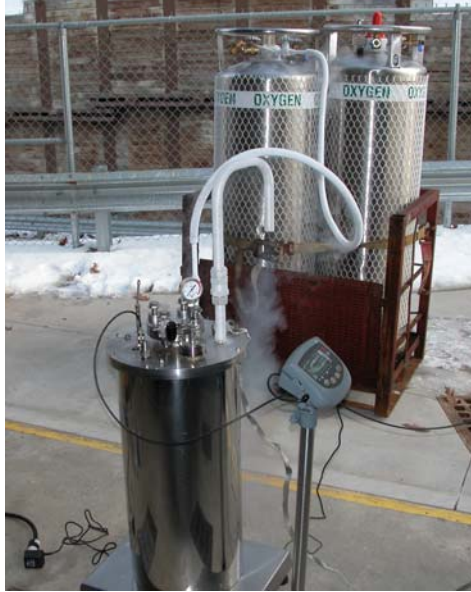
Figure 4.—The dewar was incrementally filled with liquid oxygen, and weighed using a floor scale to determine the fill level.
