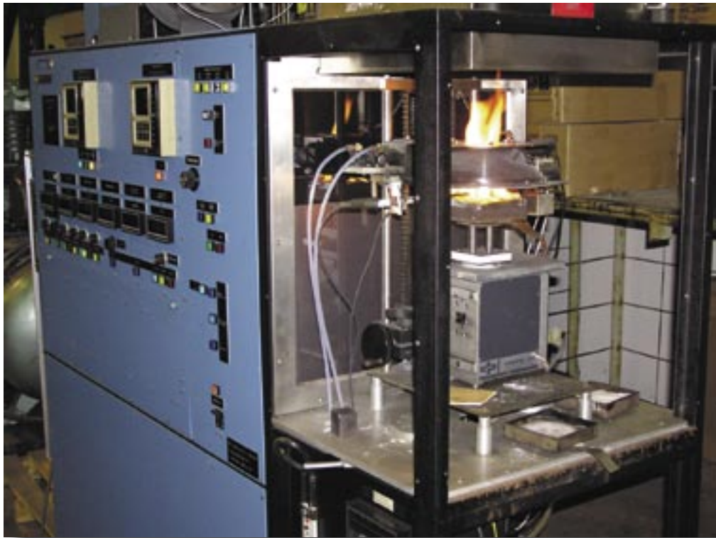
Figure 2. Refurbished cone calorimeter for studying flammability properties.
