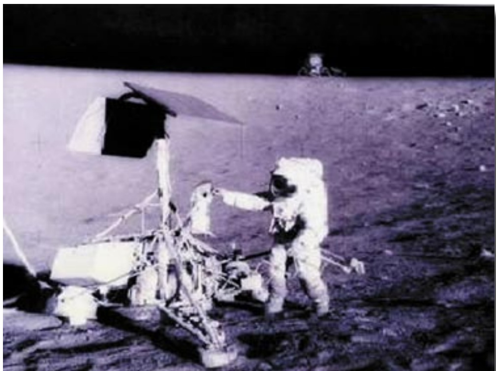
Figure 2. Apollo 12 Lunar Module landed 155 meters from the Surveyor 3 spacecraft, scouring and pitting its surface and contaminating open crevices.
