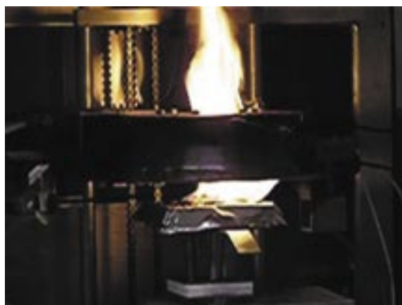
Figure 4. Cone calorimetry flammability test of 10 percent additive loading. Shown is an obvious visual decrease in size of fire compared to unmodified matrix.
