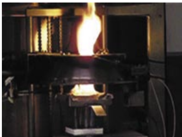
Figure 5. Cone calorimetry flammability test of 20 percent additive loading. Shown is a visual decrease in size of fire compared to 10 percent, and a significant decrease compared to unmodified matrix.
