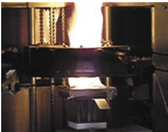
Figure 3. Cone calorimetry flammability test of unmodified matrix.
