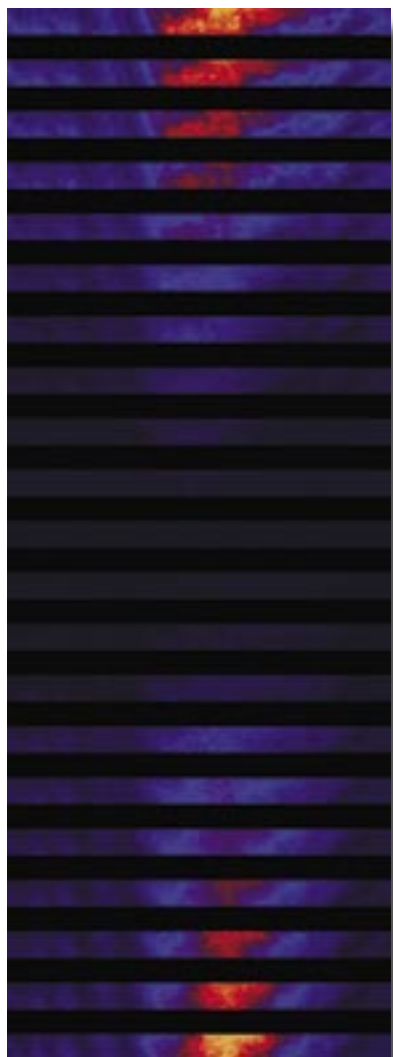
Figure 3. The response of the crystal as the voltage applied to a needle electrode is increased from -1,000 V to +1,000 V. Each slice in the image shows the same section of the crystal, with the needle electrode located in the center of the image.
