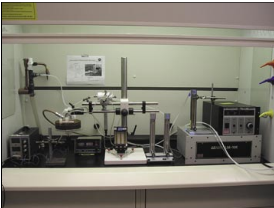
Figure 2. Plasma treatment setup.
