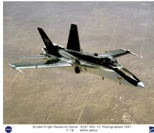
Figure 2. F-18 High Alpha Research Vehicle (HARV)
