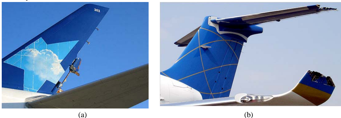
Figure 1 (a) Air Transat A310 - 2005 - Rudder Loss; (b) Embraer Legacy 600 – Brazil – Wing Tip and Stabilator Loss, September 2006.
