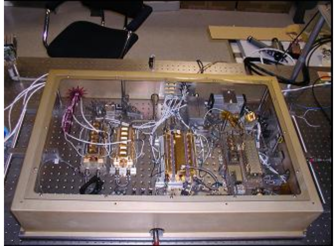
Figure 1. The final Nd:YAG pump laser assembly packages inside a box with ring laser oscillator and four amplifiers.
