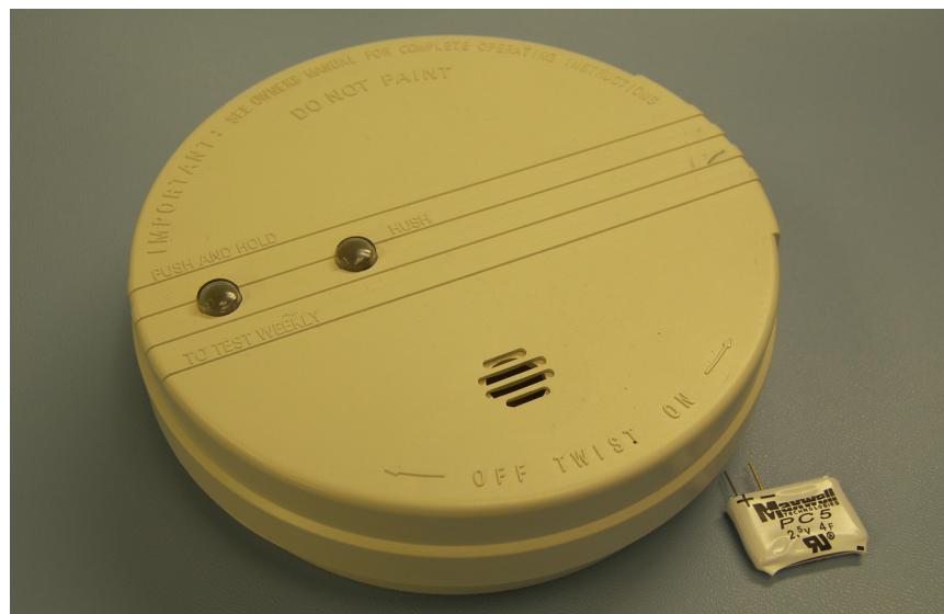
Figure 18.—A hybrid smoke alarm powered by utility ac power and ultracapacitors.
