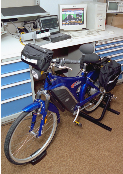
Figure 5.—A hybrid electric bicycle was tested successfully with a bank of ultracapacitors for the energy storage system.
