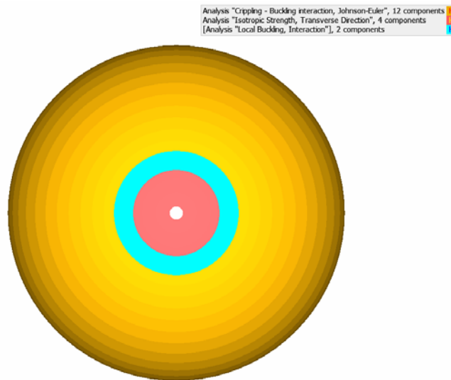
Figure 8.—Illustrates the controlling failure modes for the outer tank wall. Same result for opposite polar region.
