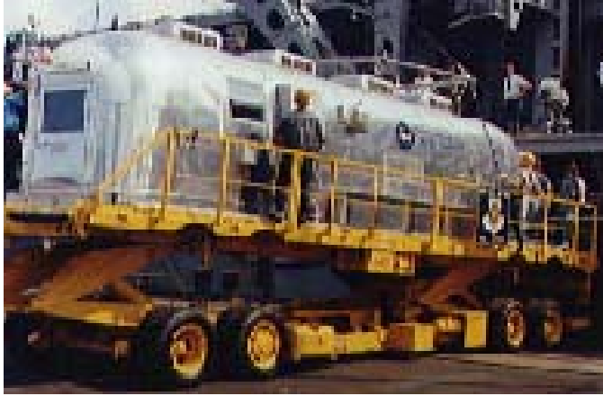
Figure 2. Mobile Quarantine Facility (MQF) used during the Apollo lunar program to transport astronauts from the splashdown sites to the containment facility in Building 37 at the Johnson Space Center. The MQF could be transported on the deck of an aircraft carrier as well as inside of an aircraft (44).
