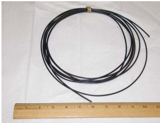
Figure 3: Extruded tubes of Elvax™ 260/nanofillers
