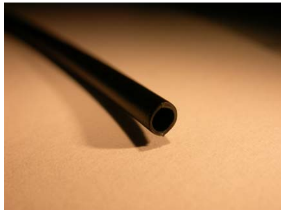
Figure 3: Extruded tubes of Elvax™ 260/nanofillers
