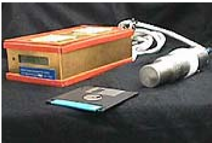
Figure 3. The Tissue Equivalent Proportional Counter (TEPC) is an automatic microdosimetry system, which consists of a spectrometer unit and a detector unit. The spectrometer unit contains a computer that allows real-time analysis of the data and provides data on the dose equivalent rate as a function of lineal energy ( y ) and time for space radiation. The TEPC is filled with a low pressure gas. TEPC's are also used in aviation.
