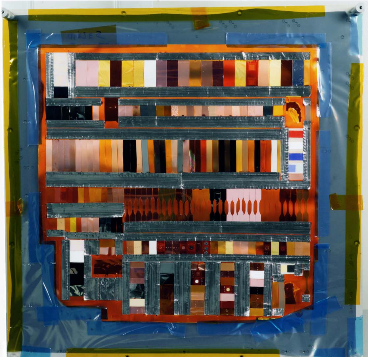
Figure 7. – Postflight photograph of MISSE 5 thin films blanket.
