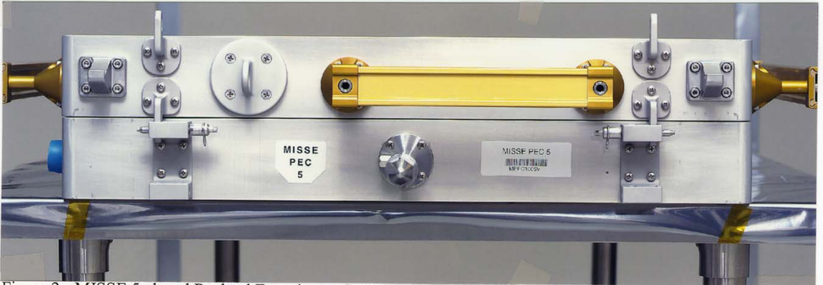
Figure 2.- MISSE 5 closed Payload Experiment Container (PEC).
