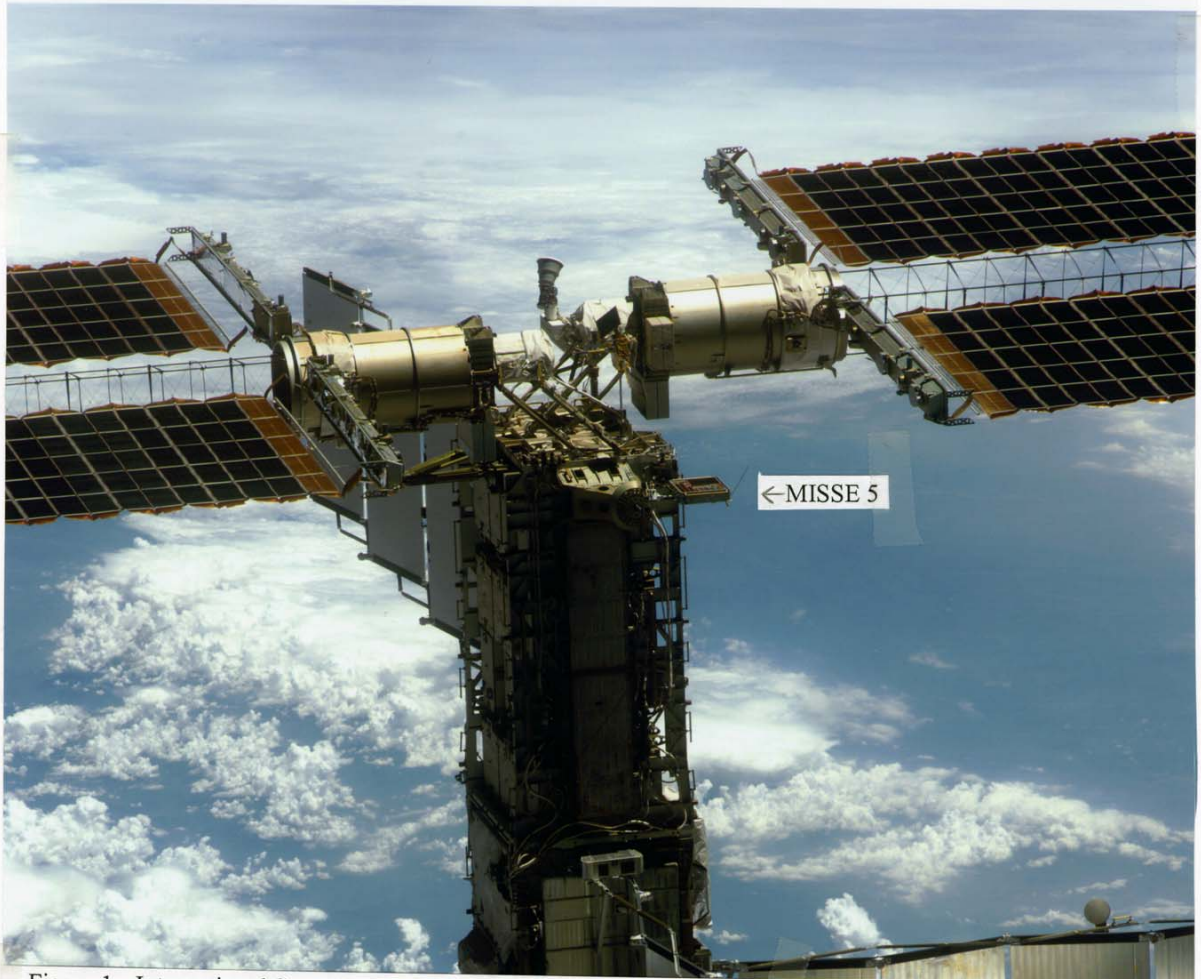
Figure 1.- International Space Station (ISS) solar arrays and MISSE 5.
