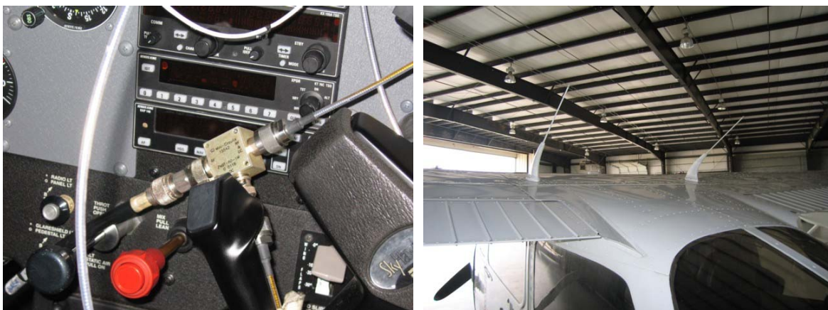
Figure 4.2-2: Powering the GPS antenna using a bias-Tee. External VHF antennas.
