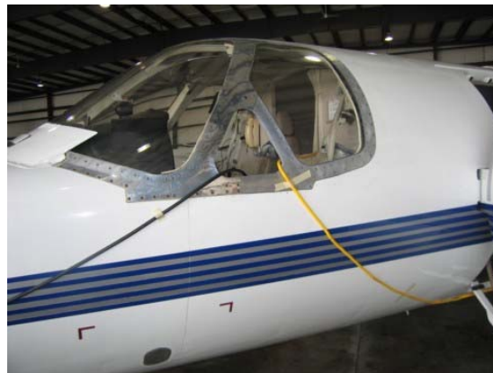
Figure 4.6-2: Cables to the outsides were taped tightly to the body to minimize re-radiation.
