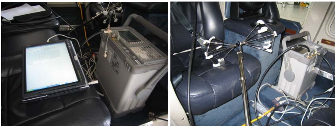
Figure 4.3-2: Spectrum analyzer and biconical antenna.
