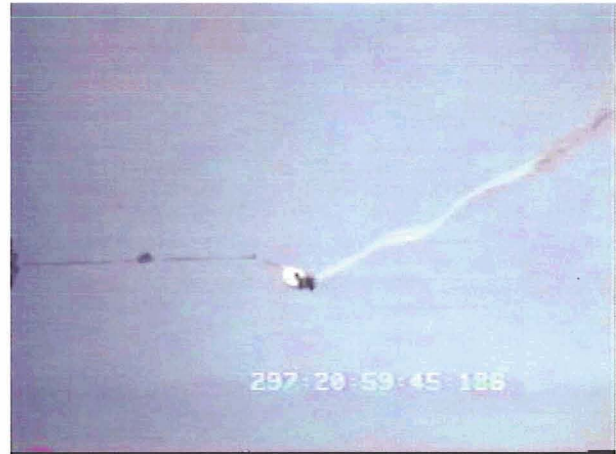
Figure 7. Large angle of attack at bag strip on test 2
