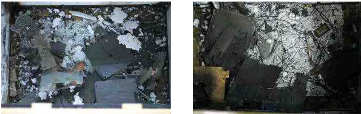
Fig. 3. Fragmentation of the target satellites: (left) low-velocity impact; (right) hypervelocity impact.
