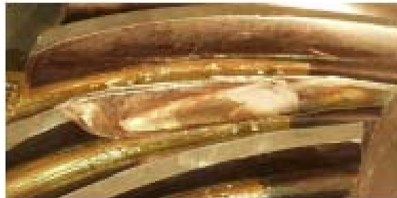
Figure 9.—Pinion cracked tooth at test completion.
