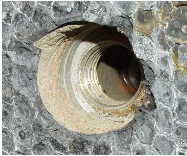
Fig. 9. Photograph of ablator plug hole on Apollo/Skylab 3 aft heat shield.
