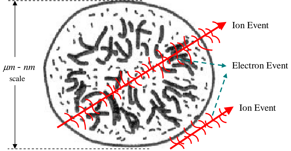
Figure 2. Schematic of ion and electron energy deposition processes within a micro-volume.
