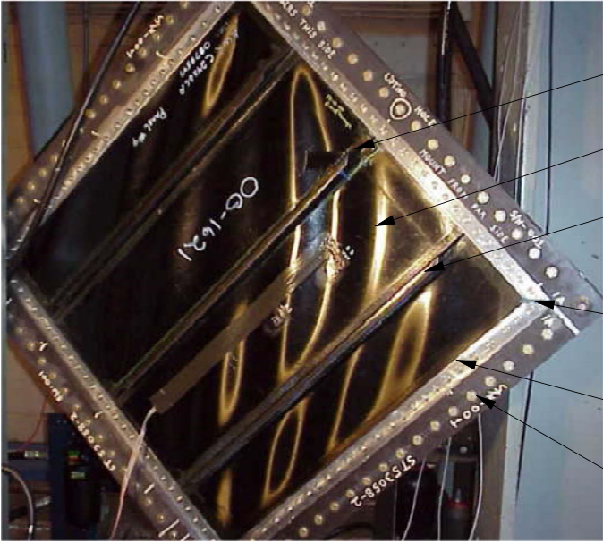
a. Buckled composite panel under shear loading with picture frame.
