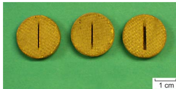
Figure 3.—Machined slots in RCC buttons. From left to right, slots have nominal widths 0.25, 0.51, and 1.02 mm, respectively.
