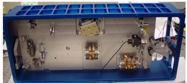
Fig. 5. Compact, rugged coherent lidar transceiver in enclosure.
