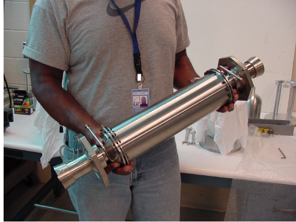
Figure 8.—TDC mass simulators attached to a common pressure vessel in preparation for vibration test.
