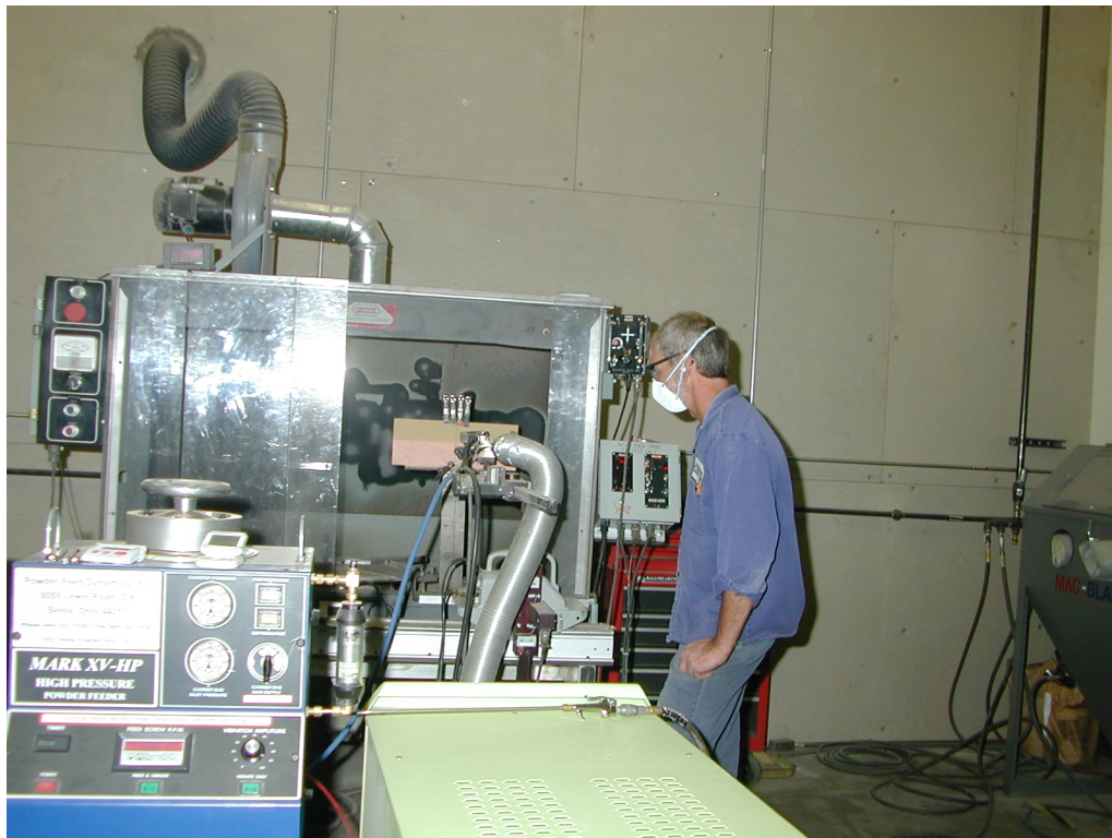
Figure 6.—Cold spray processing of plate specimens.
