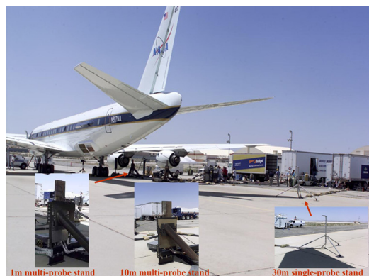
Figure 1: Photos of APEX sample stands - 1 m and 10 m stands each with a multi-probe rake, 30 m stand with a single probe
