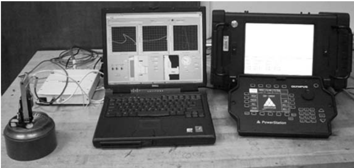
Figure 3. Complete eddy current PRCS thruster inspection system.
