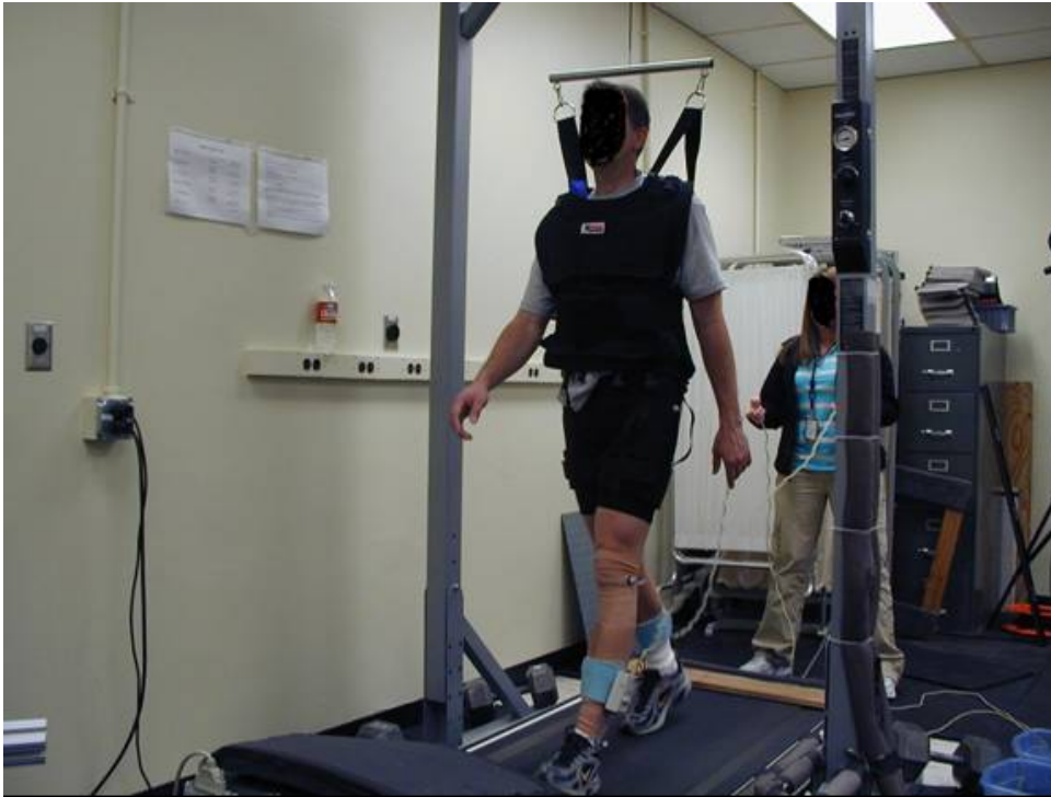
Figure 3. Typical data collection with the H/P Cosmos Airwalk Unweighting System and Weighted X-Vest.
