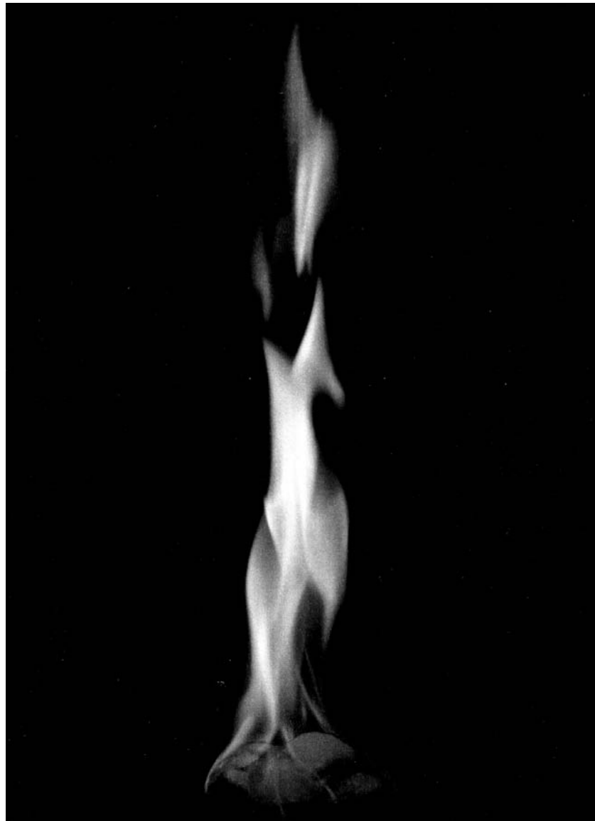
Figure 11-11. Methane ice burning (courtesy of the Morgantown, WV, USA, Energy Tech Center of the U.S. Department of Energy (1990)).
