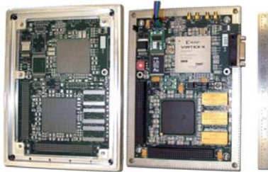
Figure 3. Reconfigurable board developed by NASA’s RSC project.
