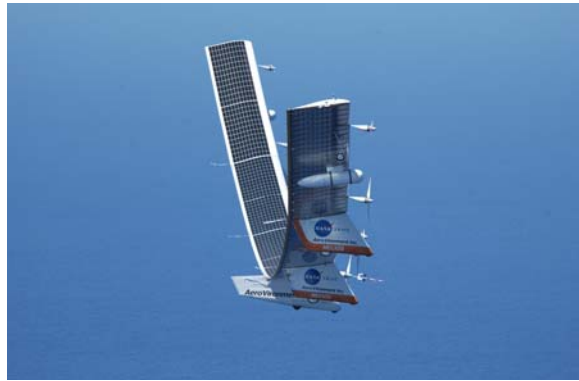
Figure 5: HP03-2 with high wing dihedral.
