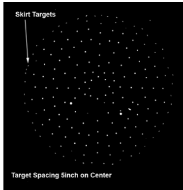
Figure 10b. Target pattern (typical) used for most drop test.
