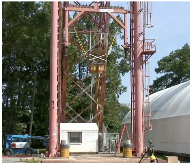
Fig. 22. Photograph of composite fuselage section suspended from the drop tower portal at the actual test drop height and a nominally flat attitude. The impact velocity was 38.4 fps.
