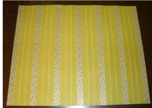
Fig. 8. Typical panel used in the fabrication of a deployable honeycomb structure showing the integrated hinge lines.
