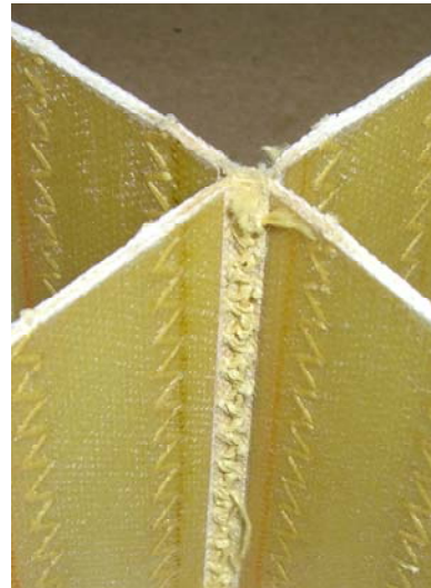
Fig. 2. Photograph of square cell junction fabricated of Kevlar 129 and E-glass fabrics. A zigzag stitch pattern was used to eliminate delamination between the glass and the Kevlar plies. The hinge is made of Kevlar 129 with the fibers oriented at \pm 45^\circ with respect to the hinge axis.
