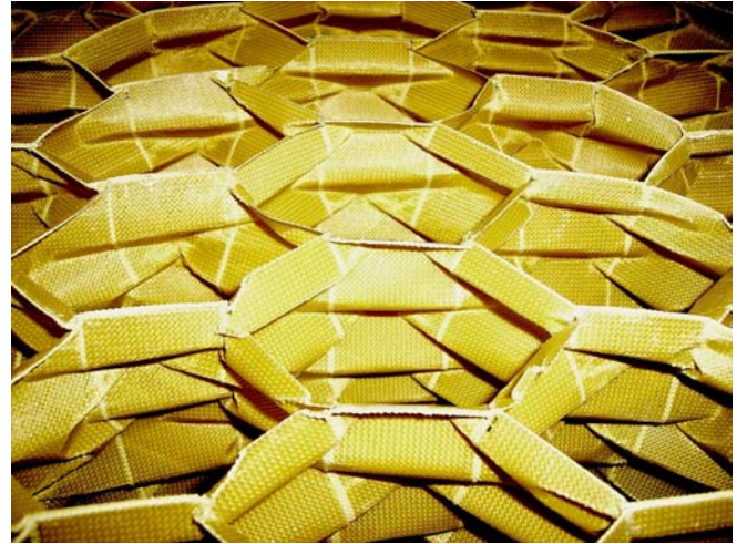
Fig. 13. Post-crush photograph of a deployable honeycomb made of Kevlar-129.
