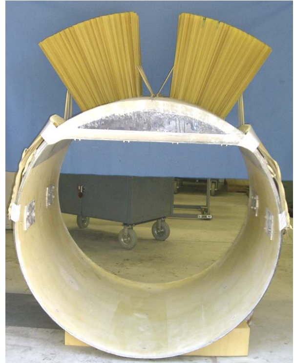
Fig. 24. Photograph of composite fuselage section with four energy absorbers: – two of the EA are shown in the packed position. The fuselage section is photographed upside down.
