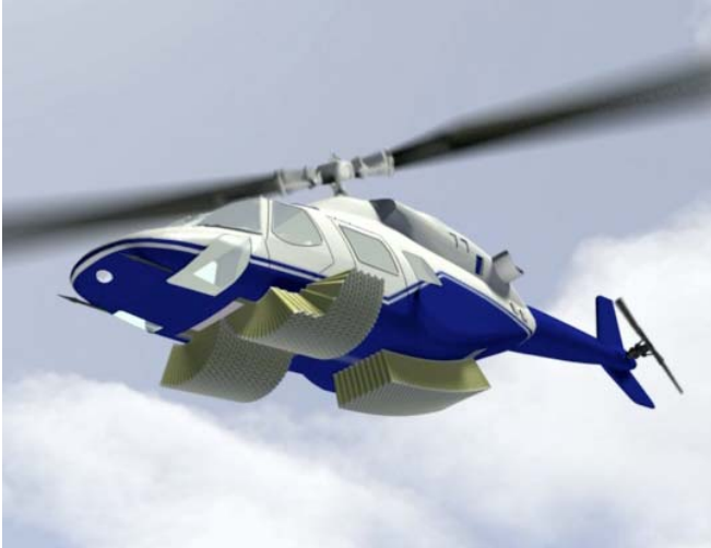
Fig. 6. Artist's rendition of a rotorcraft with a set of energy absorbers deployed. The front energy absorbers are shaped to allow for egress. The flexible cover that would normally be used to cover the outer surface of the EA is not shown.
