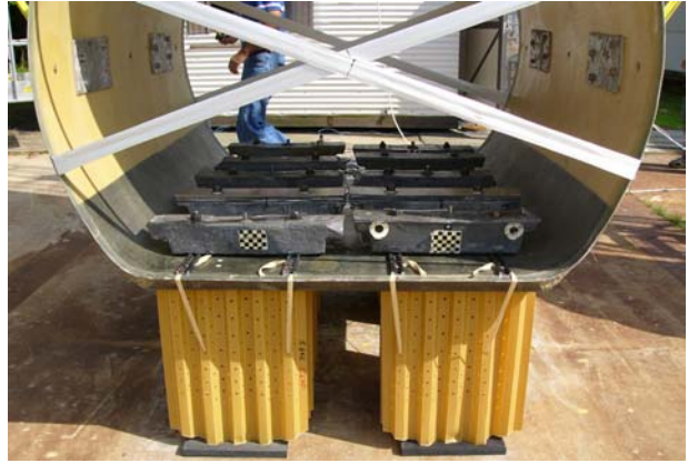
Fig. 21. Photograph of composite fuselage section with energy absorbers installed. A radius of curvature of approximately 18'' was machined in each EA to attenuate the initial peak load.
