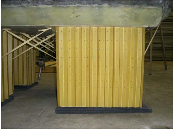
Fig. 9. EA installed on a test article in preparation for a drop test. Kevlar straps, which extend through the EA, stabilize each EA.
