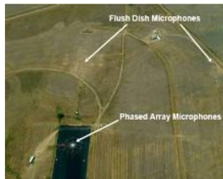
Figure 5. Layout of microphones with respect to the runway.
