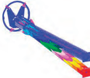
Figure 6. Detailed Mock QS mode shapes and frequencies.
