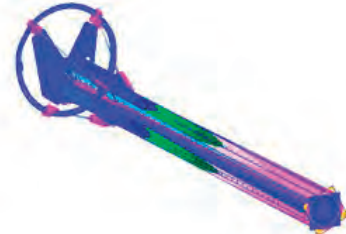
Mode 3-torsion (7.876 Hz)
