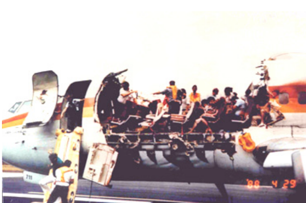
(a) Forward fuselage after Aloha Airlines accident (1 person killed)
