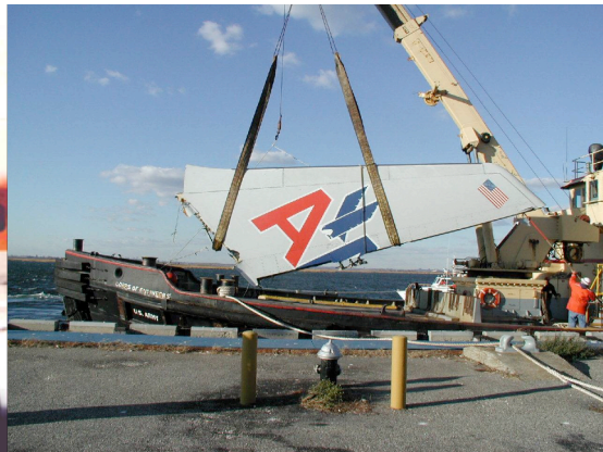
(b) Recovery of Vertical Tail after American Airlines Flight 587 accident (265 people killed)
