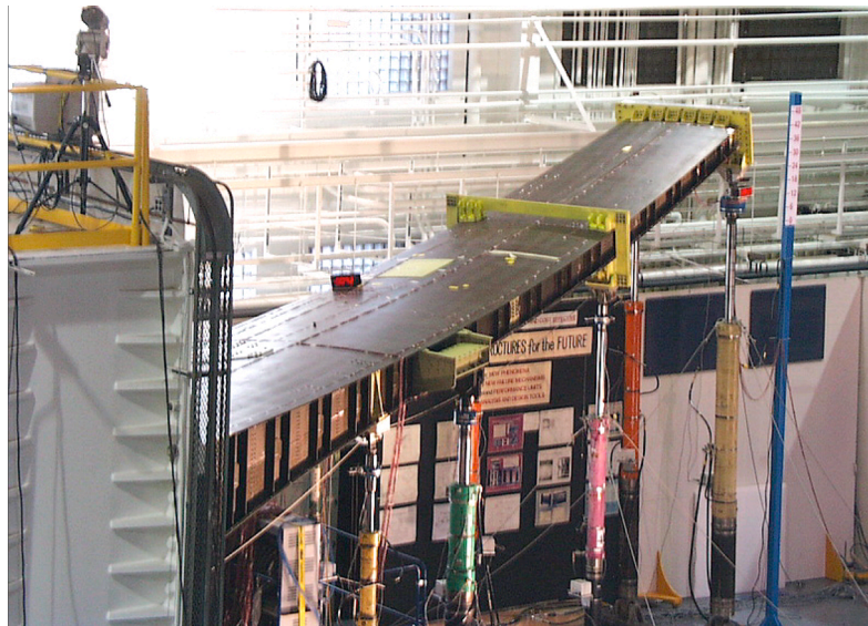
Figure 6: Ultimate Load Test of Stitched/Resin Film Infused Composite Wingbox
