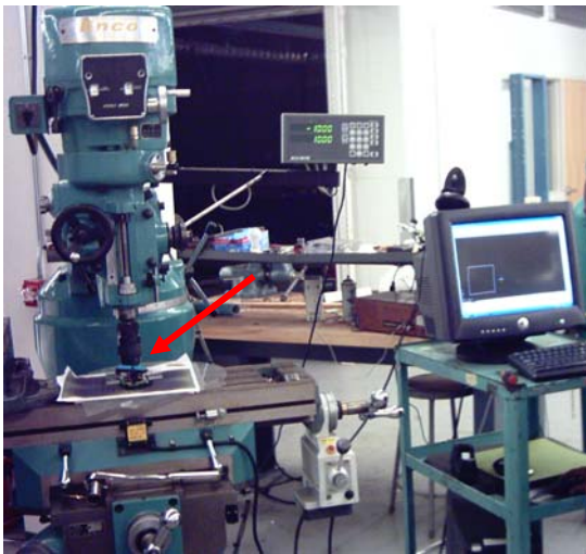
Figure 2. Laser mouse testing set up
