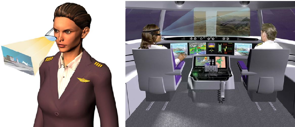
Figure 1. A Synthetic Vision enhanced HWD with a head tracker has unlimited field-of-regard.
