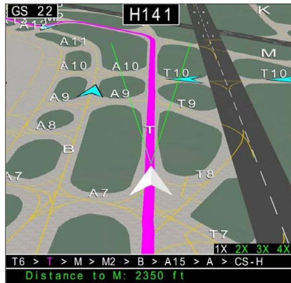
Figure 8. The Advanced EMM with traffic icons (blue chevrons), routing and clearance text.
